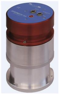
The two-dimensional inclination measurement sensors ZEROMATIC is perfectly suited for any application where monitoring of the smallest changes in absolute inclinations over a longer period of time is required. The extremely high accuracy is achieved by measuring and compensating for any drift of the absolute "zero" by applying an automatic reversal measurement at defined intervals.
