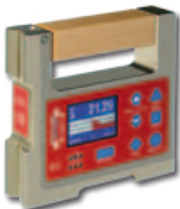
BlueCLINO with prismatic bases made of cast iron, rust protected
