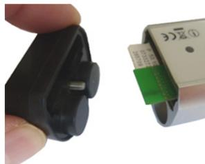
The SIM card can now be carefully inserted without applying force. Please ensure that the contact surfaces are in the correct position.
