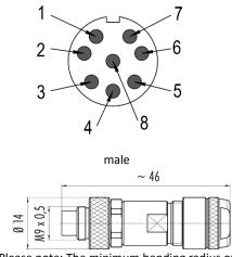
Please note: The minimum bending radius of the cable must also be taken into account
