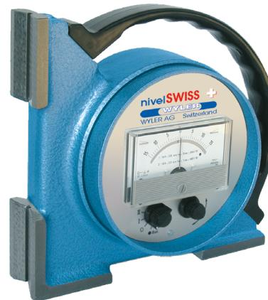
Battery powered electronic inclinometer with analog display on a built-in galvanometer. The remarkable stability of the zero-point makes this instrument particularly suitable for long-term measuring tasks and for adjustment or alignment works on large guideways. The niveLSWISS is mounted in a rugged body of carefully treated cast iron.
