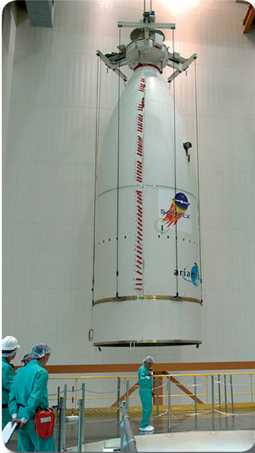
Cradle to lift and place payload fairing of an Ariane rocket
