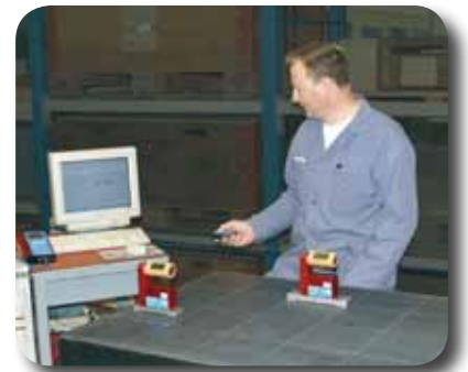
Flatness measurement with a measuring and reference instrument
