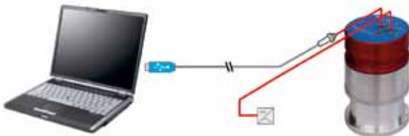
ZEROMATIC connected through a USB cable to a PC/laptop, distance from the measuring instrument to the PC/laptop max. 1.8 m
