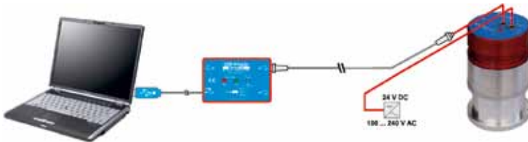
ZEROMATIC connected through an USB-Adapter to a laptop or PC, distance from the measuring instrument to the PC/laptop max. 1000 m
