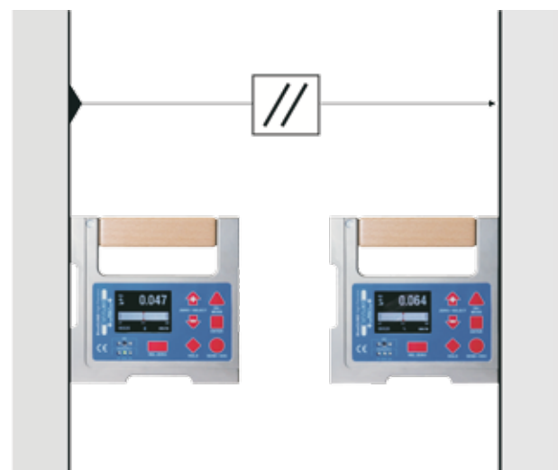
Simple comparison of a left and a right vertical guideway
