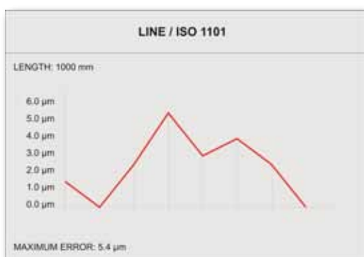
Straightness of lines with or without twist, in accordance with ISO1101
