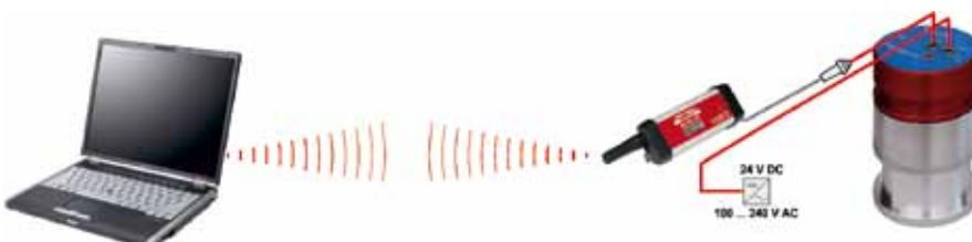
Data transmission of the ZEROMATIC device by means of a data logger. Reading the data from the datalogger into the PC / laptop via wireless data transmission.
