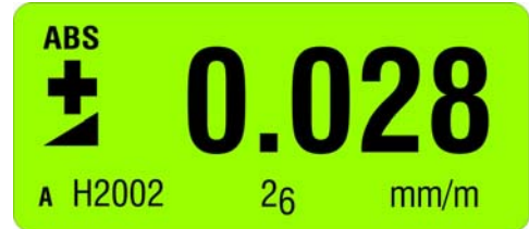
Indication with sufficient voltage U_{INT} > 4,75V
